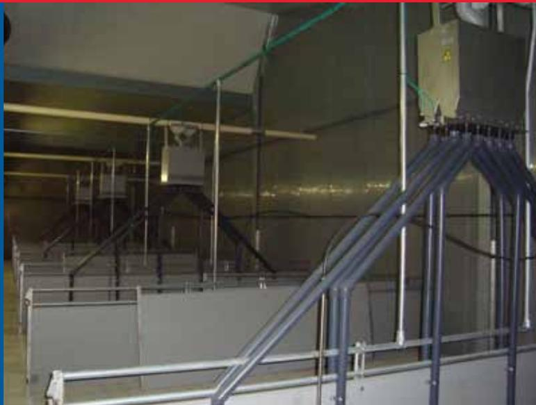
The Feed Distribution Unit is applicable to houses with sows, gilts or fatteners. It can be installed with the VDL tube feeding system or auger system. The hopper is made of stainless steel.
