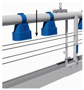
When feeding time starts the feedtrough controlled by an automatic winch is winched down to *feeding position*, so all males can eat simultaneously.
